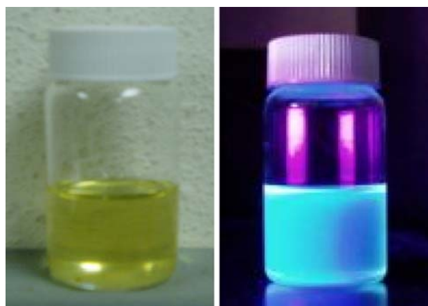
Fig. 1 Solution of synthesized ferroan sphalerite nanoparticles under (a) white light and (b) UV light from handheld emitter
